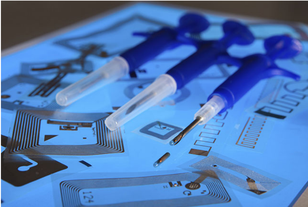
Rice grain size implants and injection tools..
